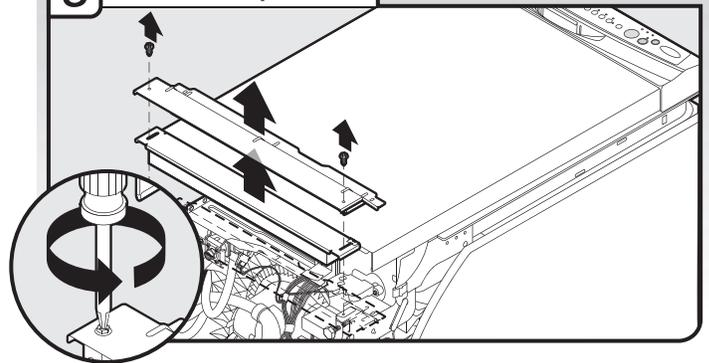
Using a 1/4" hex head socket, nut driver or Phillips screwdriver, remove the 2 screws attaching access panel and lower panel to dishwasher.
